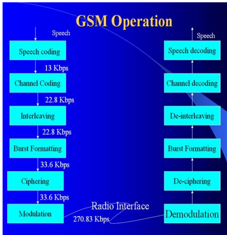
Fig -4: Operation of GSM
